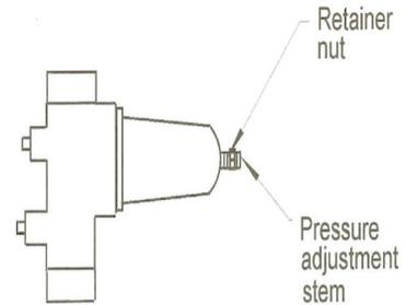
In some cases the internal components of the pressure regulator may need to be cleaned, to perform this procedure please refer to the manufactures recommended maintenance instructions or contact a licensed plumber. If you chose to perform maintenance on the pressure regulator such as cleaning of the internal seats and screens be sure to shut the water off before the regulator before you proceed.
